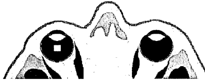
Fig. 1. Truncated human head/eye model (0.25mm resolution) with inclusion of the silicon stimulator IC model in the left eye
